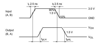
Figure 2 t<sub>pLH</sub>, t<sub>pHL</sub>
