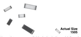
These chip resistors are available in both "top side" and "wraparound" termination styles in a variety of sizes. They incorporate self passivated, enhanced Tantalum Nitride films, to give superior performance on moisture resistance, voltage coefficient, power handling and resistance stability. The terminations consist of an adhesion layer, a leach resistant nickel barrier, and solder coating. This product will out-perform all requirements of characteristic E of MIL-PRF-55342.
