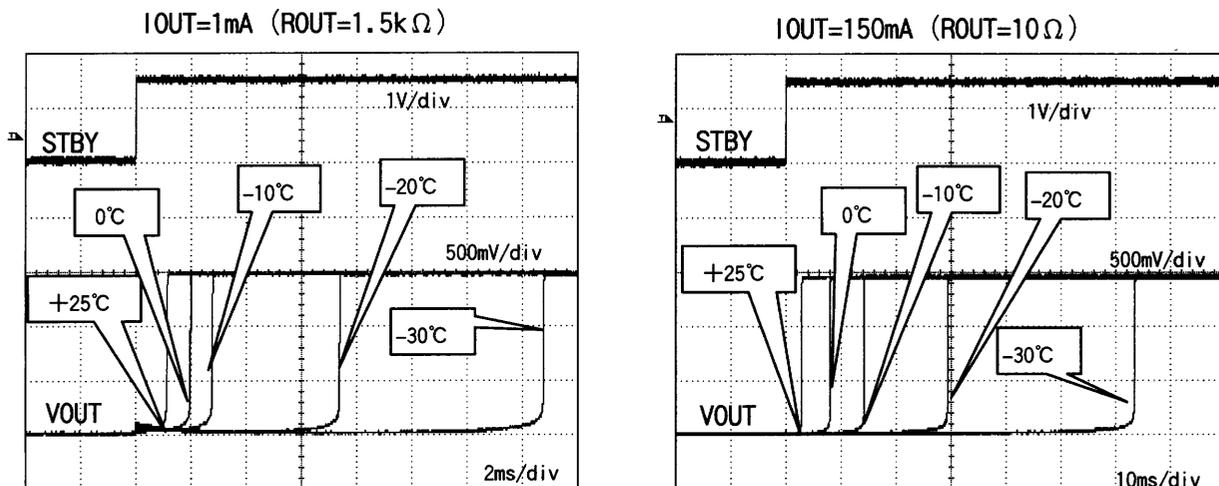
Fig. 26 Temperature characteristic of Start-up time (Reference)
