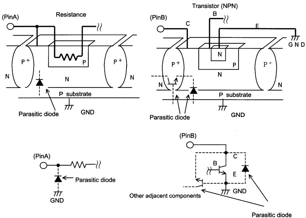
Fig.27 Simplified structure of a Monolithic IC
