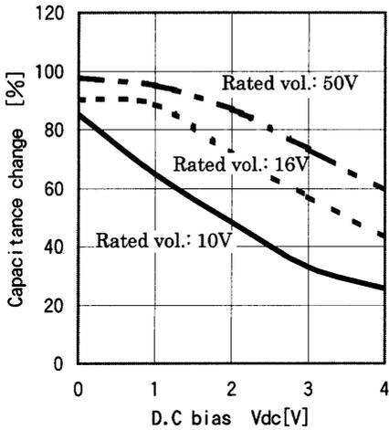
Fig. 23 Capacitance change-Bias characteristic (F type) (Reference)
