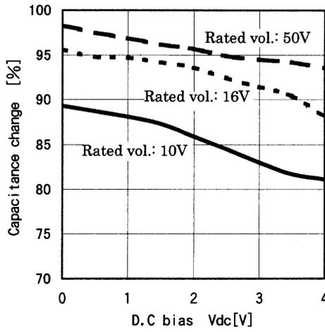
Fig. 24 Capacitance change-Bias characteristic (B type) (Reference)
