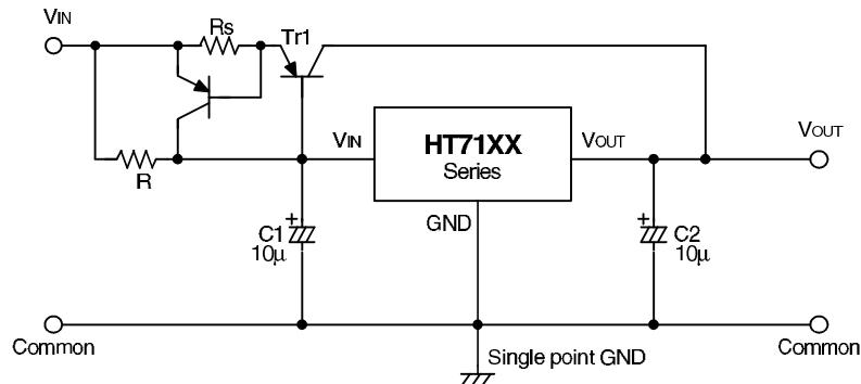
**Output voltage increasing circuit**
