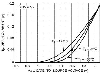
Figure 2. Transfer Characteristics
