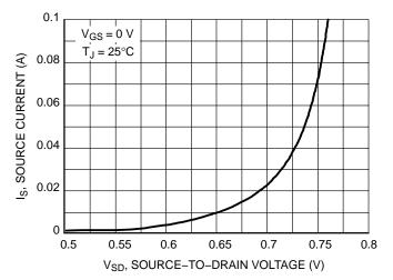
Figure 9. Diode Forward Voltage versus Current
