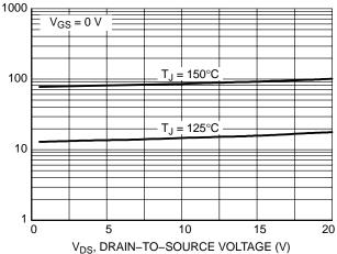
Figure 6. Drain-to-Source Leakage Current versus Voltage
