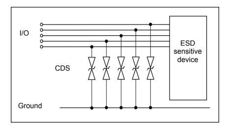
Protection of I/O Lines with discrete CeraDiodes
