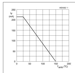
Device mounted on an FR4 printed-circuit board.
