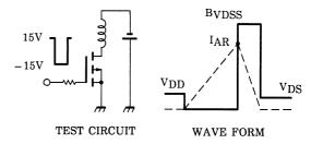
$R_G = 25\Omega$  $V_{DD} = -50V$ , L=1.44mH  $E_{\text{AS}} \!=\! \frac{1}{2} \cdot L \cdot I^2 \cdot (\frac{B_{\text{VDSS}}}{B_{\text{VDSS}} \!-\! V_{\text{DD}}})$
