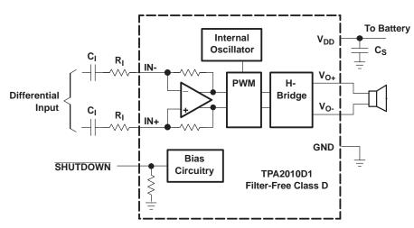
Figure 28. TPA2010D1 Application Schematic With Differential Input and Input Capacitors
