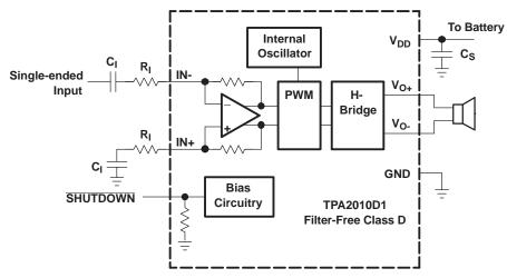
Figure 29. TPA2010D1 Application Schematic With Single-Ended Input
