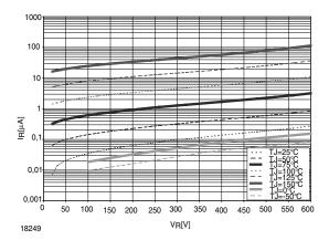
Figure 4. Typical Reverse Characteristics
