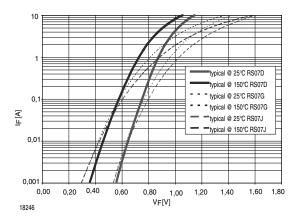
Figure 1. Typical Forward Characteristics
