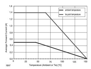
Figure 2. Forward Current Derating Curve
