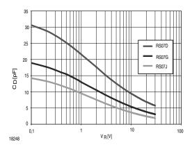
Figure 3. Typ. Diode Capacitance vs. Reverse Voltage
