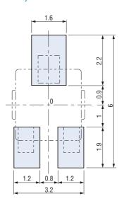
Note 1) The zero point is the center of mounting.
