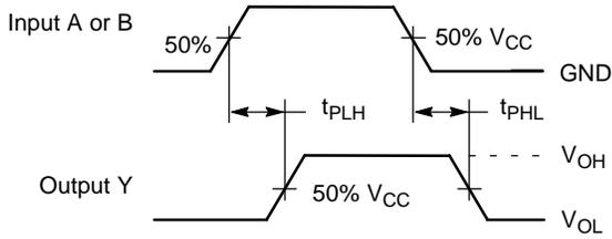
**Figure 4. Switching Waveforms**
