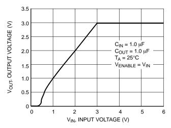
Figure 12. Output Voltage vs. Input Voltage
