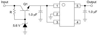
Figure 17. Input Voltages Greater than 6.0 V
