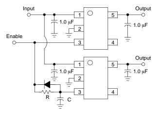
Figure 16. Delayed Turn-on
