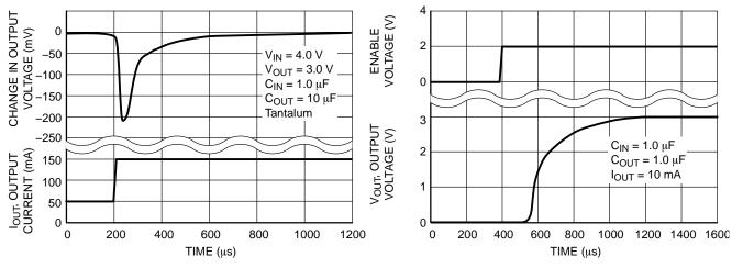
Figure 10. Load Transient Response
