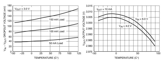
Figure 2. Dropout Voltage vs. Temperature
