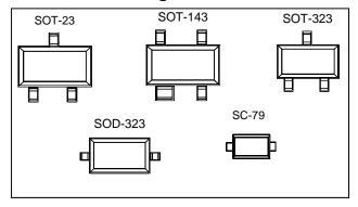
The diodes are come in various chip configurations and are available as single diodes, series tees (ST), series tee reverse (STR), common cathode pairs (CK), common anode pairs (CA), and unconnected pairs in the respective featured packages.
