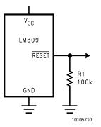
FIGURE 1. **RESET** Valid to  $V_{cc}$  = Ground Circuit
