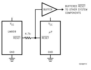
FIGURE 3. Interfacing to Microprocessors with Bidirectional Reset I/O
