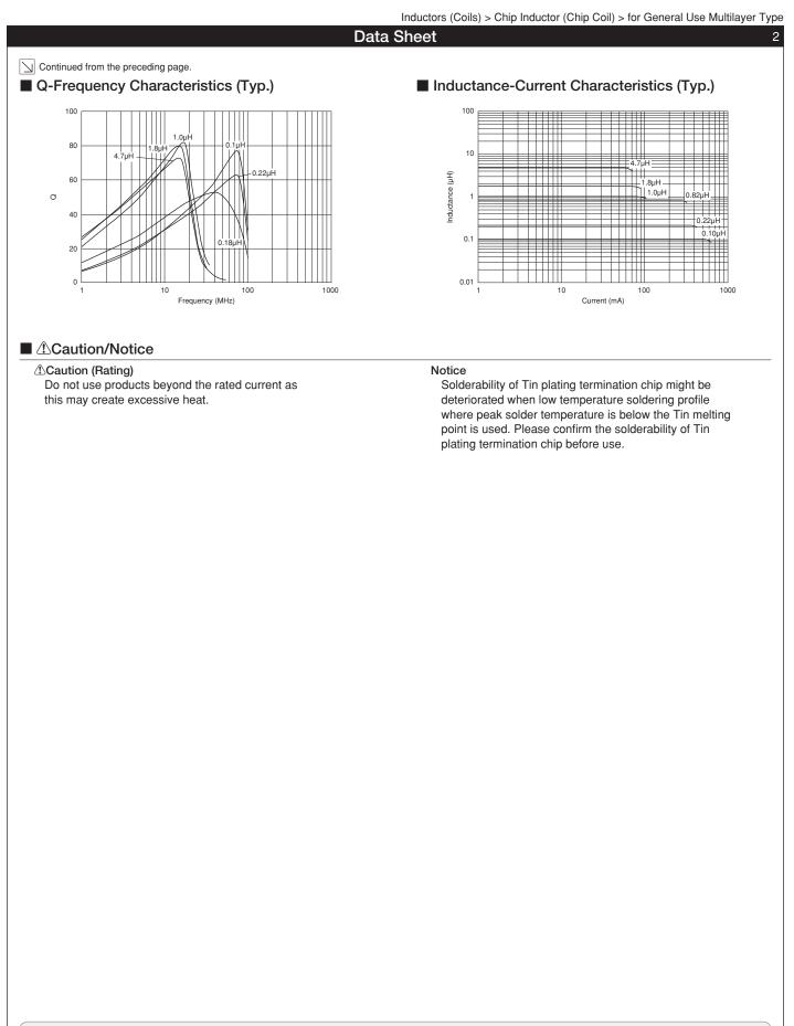
•This data sheet is applied for CHIP INDUCTORS (CHIP COILS) used for General Electronics equipment for your design.
