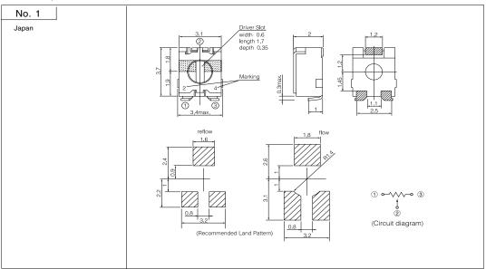
Note: Mounting not possible after trimming knob has been rotated.
